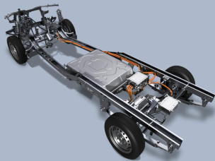
The battery is designed in an embedded manner
